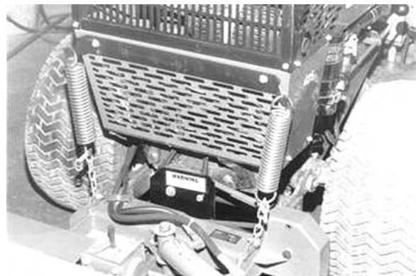
Photo 2 - Hose Clamp and Routing
